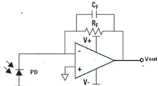
Figure 1: Transimpedance amplifier circuit
