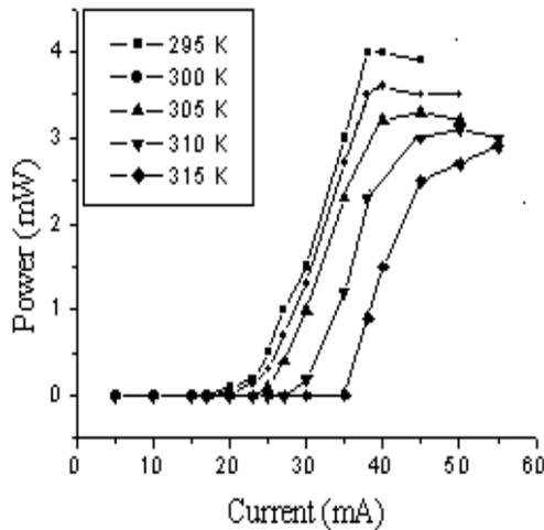
Figure 3: The Optical output power vs. driving current characteristics at different temperature
