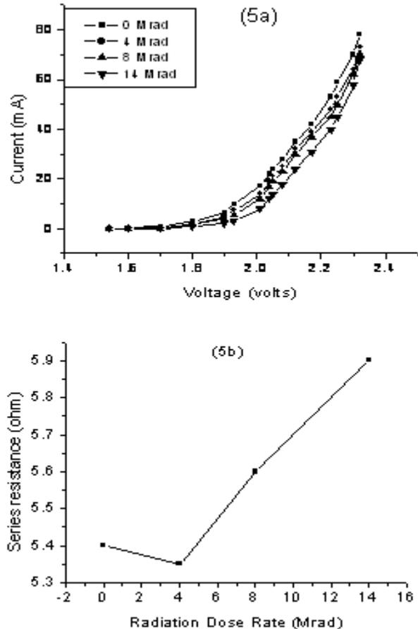
Figure5: The direct voltage vs. the driving current a) and the change of series resistance b) for different total irradiation dose
