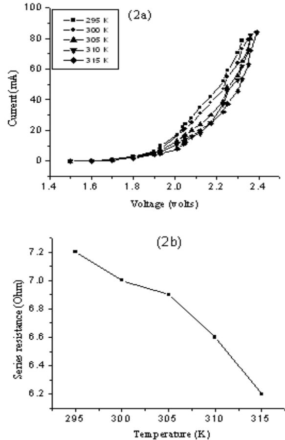
Figure 2: The direct voltage vs. the driving current characteristics a) and change of serial resistance b) at different temperature
