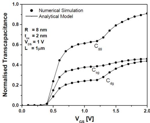
Fig.6. Comparison of normalized transcapacitances obtained from our analytical model and numerical simulations using capacitance equations in [2].
