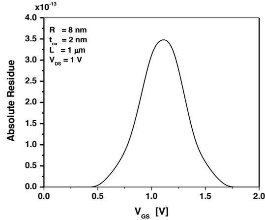
Fig.3. Plot of absolute residue in  $\beta$  values, obtained from plugging the results from our analytical model in (3), in [4]
