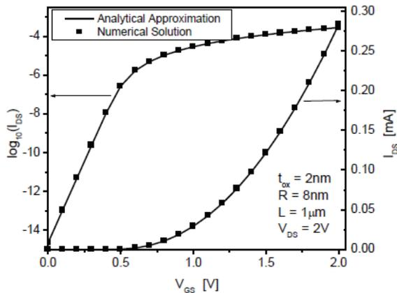
Fig.5. Comparison of  $I_{DS}$  (both log and linear scale) as obtained from surface potential values calculated numerically and from our analytical solution for different  $V_{GS}$  using equations in [2].
