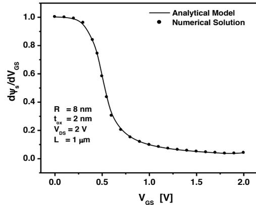
Fig.4. Comparison of first derivative of surface potential obtained from the analytical solution for different values of  $V_{GS}$ , with that from numerical solution.
