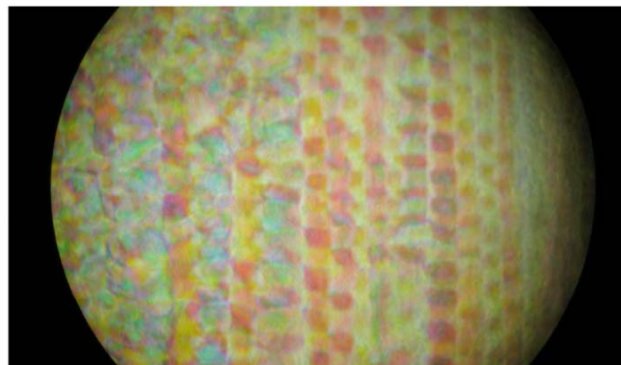
Figure 4: optical microscopic image of NCC solid thin films. Note the square formations.
