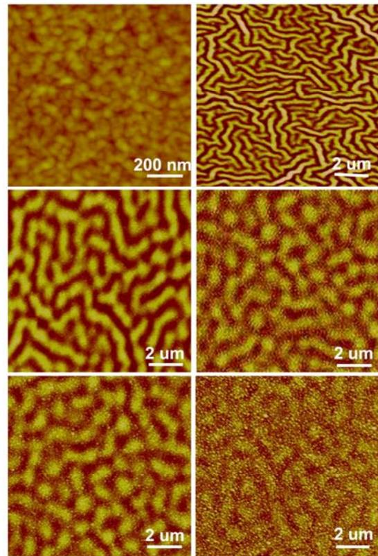
Figure 2: Wrinkles of different Sn film on 56 nm PS. The Sn films are deposited for 60(a), 100(b), 200(c), 300(d), 400(e) and 500(f) s. The wrinkles were fabricated by annealing the samples at 120 °C for 2 h. The color scale is 50 μm.
