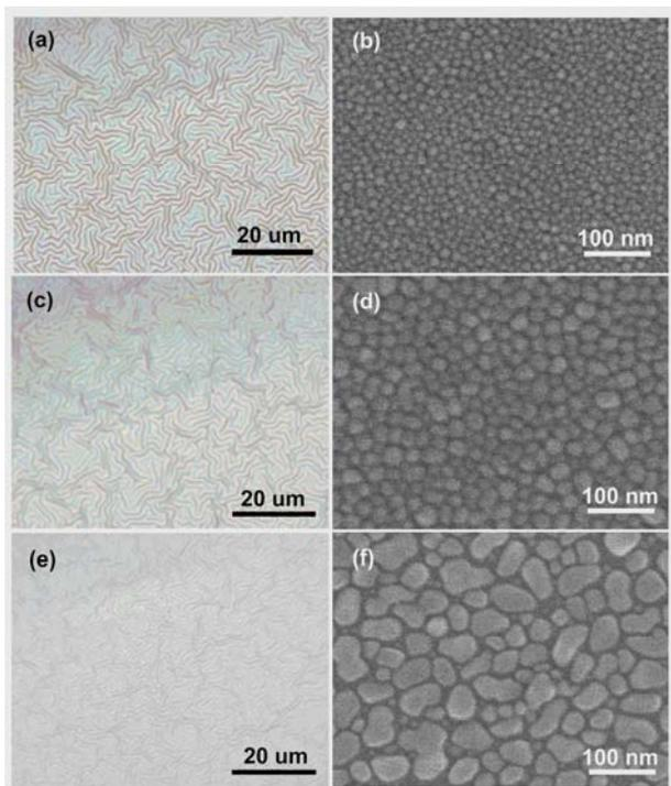
Fig. 5: The influence of film morphology on wrinkle patterns: (a), (c), (e) wrinkle patterns of 20 nm Sn film on 310 nm PS film after heating at 120 °C for 4 h. (b), (d), (f), the film morphology of Sn film in (a), (c), (e) respectively.
