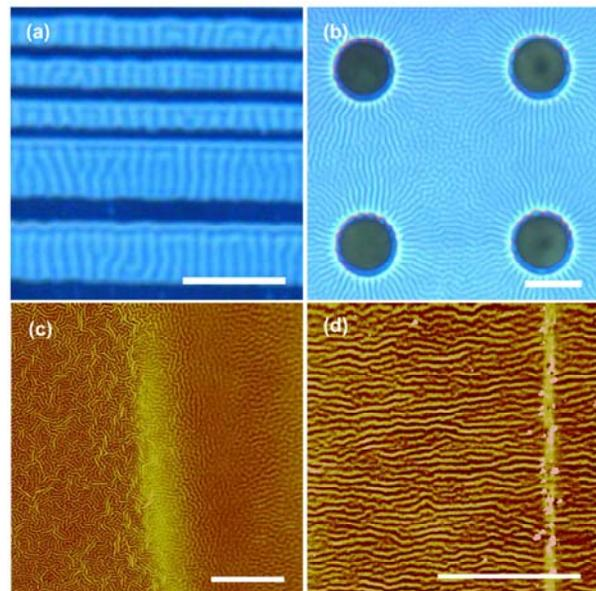
Figure 4: OM images (a, b) and AFM images (c, d) of wrinkle patterns assembled by various method. The scale bar is 5  $\mu\text{m}$ .
