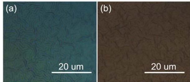
Figure 1: OM images of wrinkles of 20 nm Bi (a) and Sn (b) on 120 nm PS film. The wrinkles were fabricated by annealing the samples at 120 °C for 2 h.
