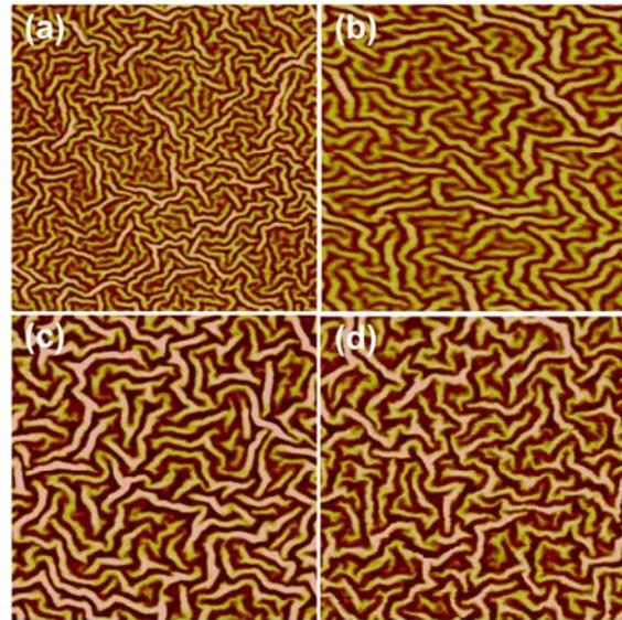
Figure 3: AFM images (5  $\mu\text{m}\times 5\ \mu\text{m}$ ) of wrinkles on 5 nm Sn film supported on different PS films. The thicknesses of PS films are 23 nm (a), 56 nm (b), 71 nm (c), 165 nm (d). The color scale is 50  $\mu\text{m}$ .
