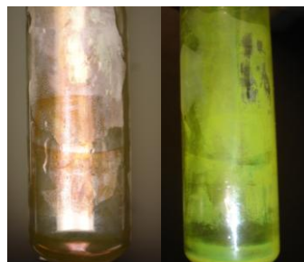
Figure 2: Colour effect of \text{Cu}_2\text{O} nanocrystals in transmitted light (left) and reflected light (right).
