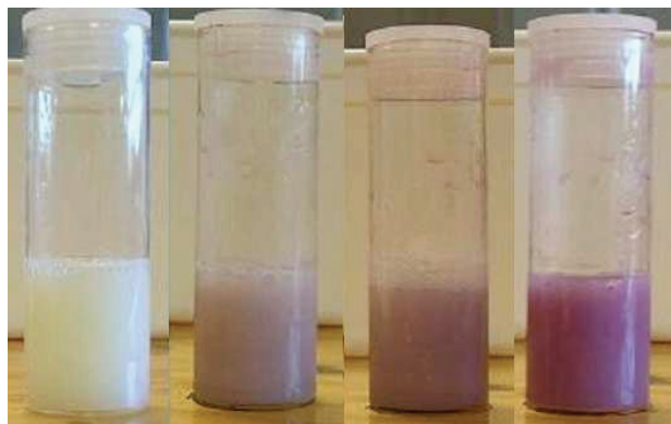
Figure 3: Polyurethane paint with increasing reaction time.
