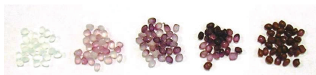
Figure 1: Polyurethane with increasing nanogold content.
