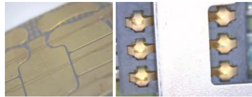
Fig 7: Optical micrographs of the super-hydrophobic film which has been scraped away by the contacting barbs of the connector. The surface tension keeps the connecting pads from being wetted by liquids.
