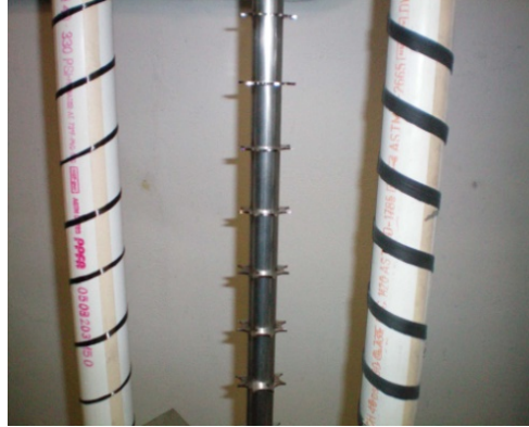
Figure 3. Electrode configurations of nanocomposite tapes wrapped on a polymer tube. The steel electrode in the center is designed on the basis of a commercial discharge electrode.
