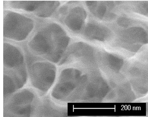
Fig. 5: SEM photograph of the nanostructured titania (NST) on the high aspect ratio bulk Ti pillars. Such nanostructured surfaces covers all the pillar surfaces and the bottom floor surface.
