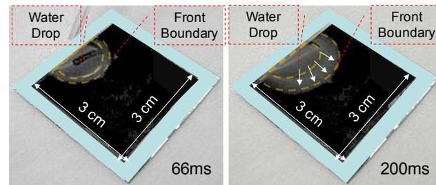
Fig. 6: Hemiwicking material was tested by placing a drop of water ( $14 \mu\text{L}$ ) at one edge of the wicking substrate. The inside half circle shows the drop forms a reservoir for the hemiwicking flow, and the outside half circle shows the front boundary of the liquid film. The drop completely wetted the nano/micro structured surface at the end, and the contact angle goes to zero.
