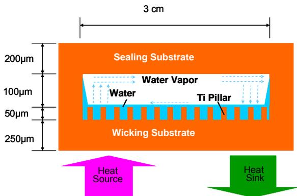
Fig. 3: Schematic of the Ti-based heat pipe. The overall device is less than 1 mm thick. The micro pillar arrays are super hydrophilic and form the wicking material.
