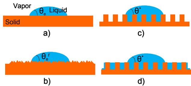
Fig. 1: a) Droplet on a smooth and flat surface; b) droplet on a practical rough surface; c) the triple line is pinned on islands; d) corresponding to film regime in which the micro/nano structures outside the drop is filled with a liquid.
