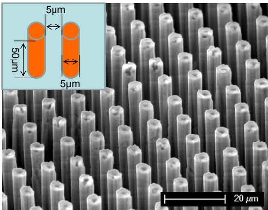
Fig. 4: SEM photograph of the high aspect ratio bulk Ti pillar arrays. The height of the pillars is about  $50 \mu\text{m}$ .
