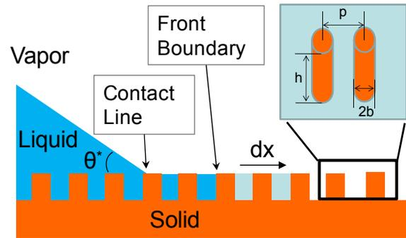
Fig. 2: Flow of the impregnating film at the front boundary. The precursor film was formed by a molecular liquid layer. As it progresses by  $dx$  and coat the nano/micro structured surfaces, it replaced the solid-air surface energy by with the solid liquid energy. A negative energy change takes place, and complete wetting is formed with this progression.
