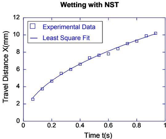
Fig. 7: This plot shows the capillary flow front boundary path as a function of time. Water was used as a working fluid. As shown the front boundary travels ~10mm within 1 second.
