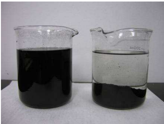
Figure 1 CNT/acetone solution dispersed by a microfluidic process (left) and ultrasonication (right)
