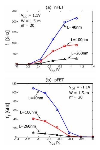
Figure 9: Cut-off frequency  $(f_T)$  vs.  $V_{GS}$  curves for (a) nFETs and (b) pFETs, each at three different gate lengths (L = 40nm, 100nm, and 260nm).  $W=1.5\mu$ m, nf=20 and  $|V_{DS}|=1.1$ V. It is clear that the model results (solid lines) well match the measurement data (symbols) at a broad range of device geometries and voltage biases.
