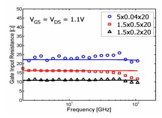
Figure 5: Measured (symbols) and simulated (solid lines) effective gate input resistance,  $Re\{(1+S11)/(1-S11)\}$ . 50 $\Omega$ , vs. *Freq.* for nFETs at three different geometries (*W/L/nf*).
