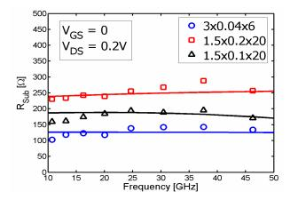
Figure 4: Extracted  $R_{sub}$  vs. *Freq.* curves for nFETs at three different sizes (*W*/*L*/*nf*). The symbols are for hardware data and the solid lines for the model results.
