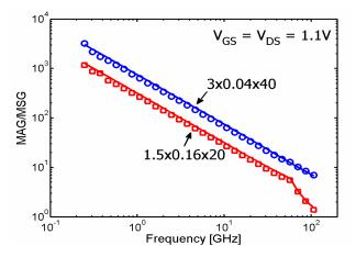
Figure 7: Maximum Available Gain (MAG) or Maximum Stable Gain (MSG) vs. *Freq.* for nFETs at two different sizes (W/L/nf). The symbols are for hardware data and the solid lines for the model results.
