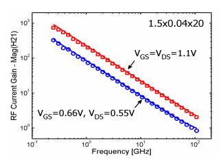
Figure 8: RF current gain, Mag(H21), vs. *Freq.* curves for a 1.5x0.04x20 (*W*/*L*/*nf*) nFET. The symbols are for hardware data and the solid lines for the model results.
