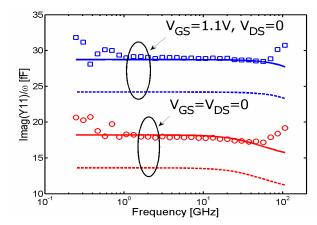
Figure 3: Gate input capacitance,  $Imag(Y11)/\omega$ , vs. *Freq.* curves for a 1.5x0.04x20 (*W/L/nf*) nFET. The symbols are for hardware data, and the solid (dash) lines are for the simulation results with (without) the wirecap model enabled.
