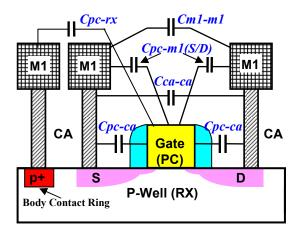
Figure 1: Wirecap network to be modeled.
