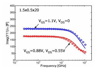
Figure 6: Measured (symbols) and simulated (solid lines) gate input capacitance,  $Imag(Y11)/\omega$ , vs. *Freq.* for a *L*=0.5µm nFET under two biases. The non-quasistatic (NQS) effect is observed and properly modeled.
