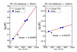
Figure 2: Measured *Cgs* vs. No. of CA curves for 3x0.04x60 (*W/L/nf*) nFETs with two different PC-CA distances, 40nm (left) and 130nm (right). The *Cpc-ca* (per CA) values can be extracted from the slopes of the two dashed lines as 0.008fF and 0.001fF, respectively.
