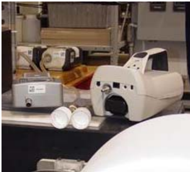
Figure 1: The nanoparticle emission assessment technique consists of an optical particle counter, 2 filter samples and a condensation particle counter.
