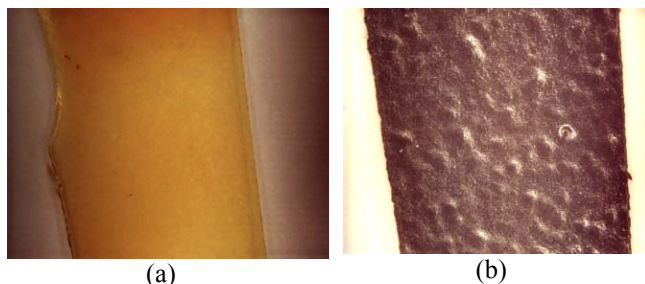
Figure 2. Stereo images of pure PI film, (a), and 10% v/v ferrite nanocomposite film, (b).
