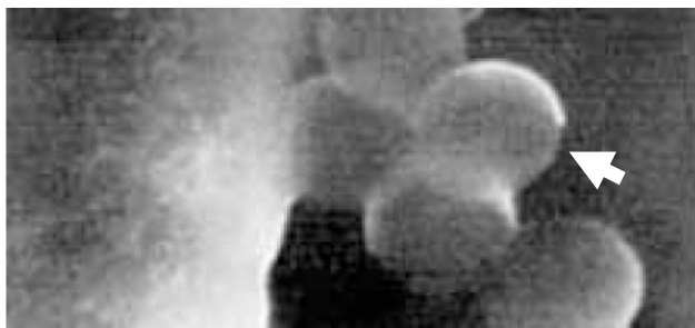
Figure 2(b): Micrograph (x 50,000) shows image with no jagged edges and no mechanical vibration. [1]
