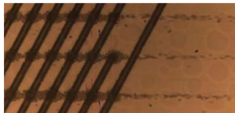
Fig. 6. Continuous enrichment of viable yeast at 20 \mu\text{l}/\text{min} with a polarized CarbonDEP array at 1 MHz and 10 V_{pp} . Medium conductivity of 51 mS/m.
