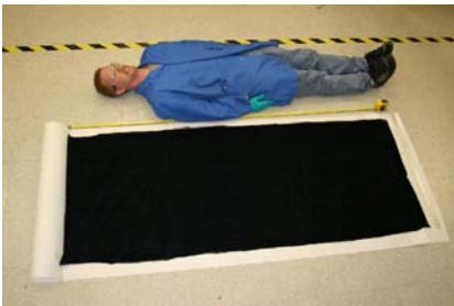
Figure 4. A >6 foot, DWCNT textile compared with a standardized “furnace operator” for scale.
