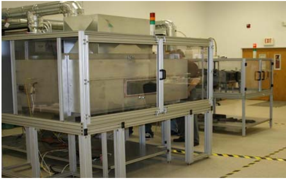
Figure 3. Apparatus to synthesize DWCNT sheets is shown above. The sheets are formed by nanotubes exiting the reactor not shown, and impinging on the belt located within the large box enclosed within the exhaust hood. The Allen Bradley controller is also not shown.
