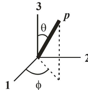
Figure 2: Definition of fiber angles
