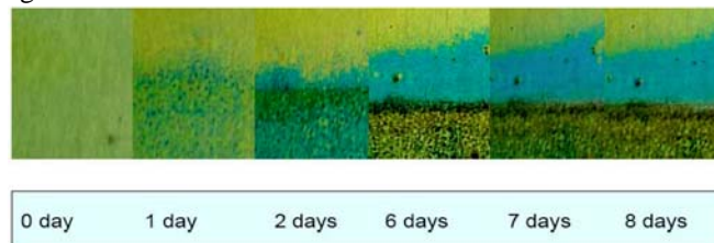
Figure 3. Results of i-clay Smart Coating in Accelerated Corrosion Test
