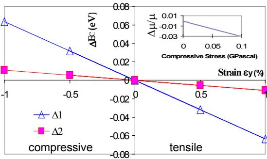
**Fig. 5:** Shift of the conduction band edge under a uniaxial stress applied along the  $W$  direction for the  $\Delta 1$  valleys of the (001) plane and for the  $\Delta 2$  valleys. Inset: the related mobility reduction.
