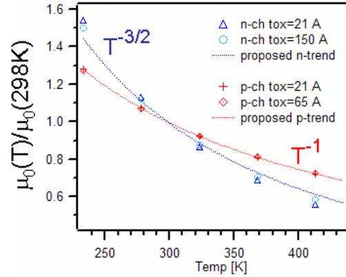
Fig. 4: Normalized temperature trend of low-field mobility for both  $n$ - and  $p$ -channel showing unchanged trend considering different technologies
