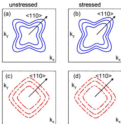
**Fig. 6:** a) Relaxed Silicon: isoenergy surface plot of the Heavy Holes (HH) at 10,20,30 meV with respect to the top of the valence band b) Compression of 1 Gpascal along the  $W$  direction; the band structure of HH are shifted and modified, reducing the mobility. c) Light Holes band, relaxed silicon; d) Same compression of b) for LH
