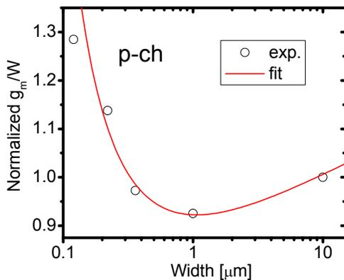
**Fig. 9:**  $p$ -channel normalized ratio of  $g_m/W$  as a function of  $W$  showing two regimes: decreasing for STI stress and increasing for  $\Delta W$ . A good match with the proposed dependence.
