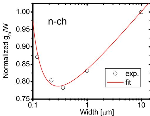
**Fig. 8:**  $n$ -channel normalized ratio of  $g_m/W$  as a function of  $W$  showing two regimes: decreasing for STI stress and increasing for  $\Delta W$ . A good match with the proposed dependence.
