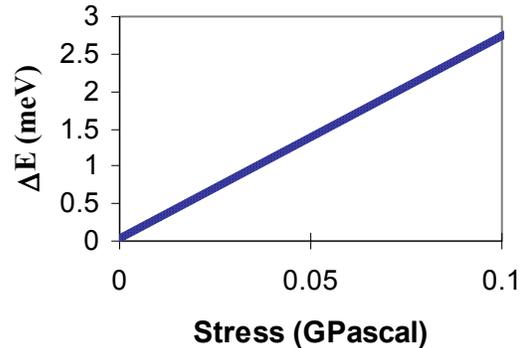
**Fig. 7:** Energetical separation between the top of the HH and the LH bands under a uniaxial stress applied along the  $W$ . The hole mobility reduction cannot be explained only by this phenomena
