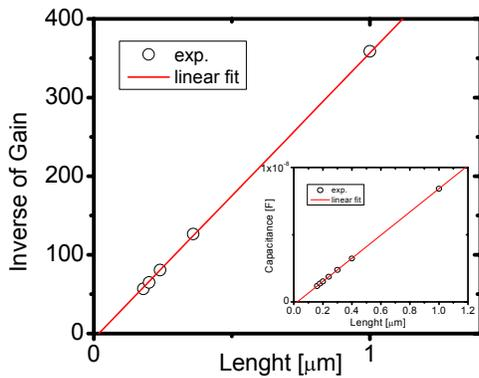
Fig. 3: Extracted  $\Delta L$  parameters from both STI-stress free structures and C-V method.
