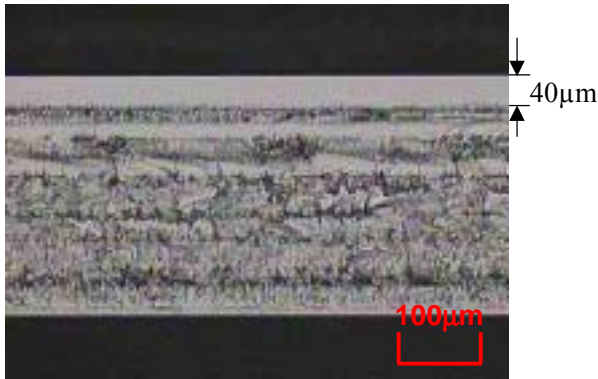
Figure 2: Edge view showing multiple SD layers.
