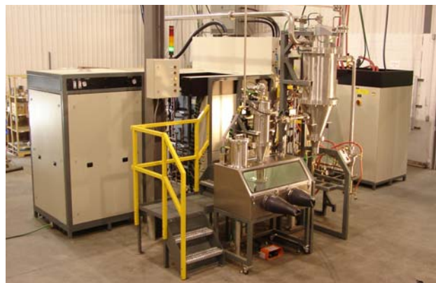
Figure 5: Typical 60 kW plasma unit commercialized by Tekna for laboratory-scale nanopowders synthesis. The nanopowder produced in the reactor is carried up to the secondary filter mounted on a glove-box, allowing safe nanopowder collection and handling and packaging under inert environment without interrupting nanopowder production.
