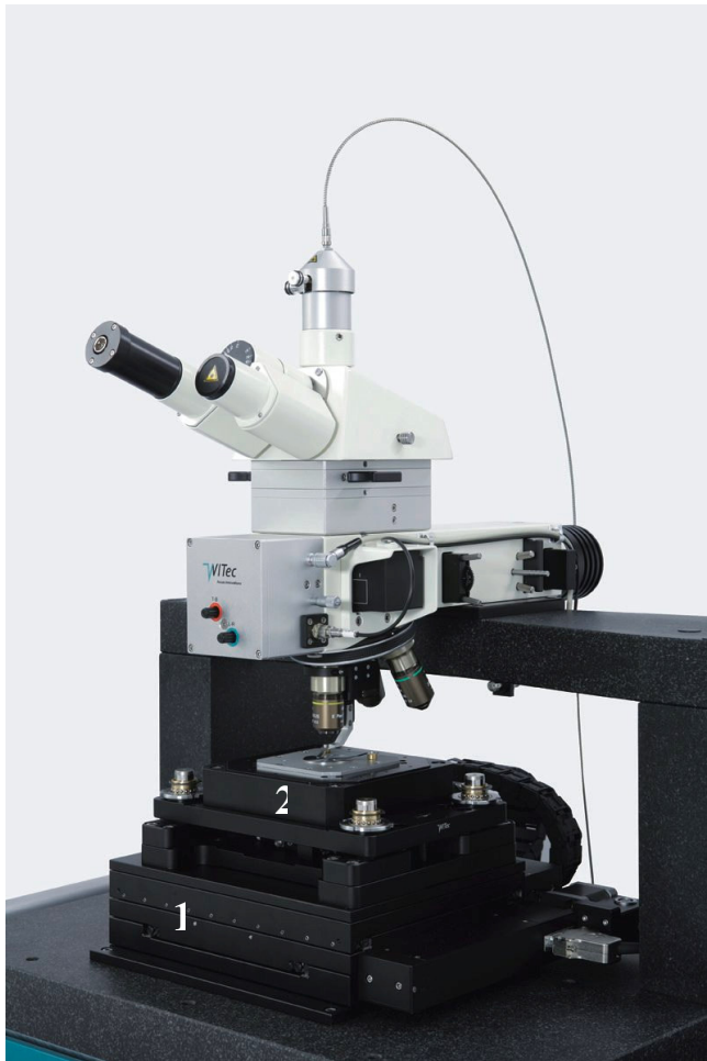
Fig. 1: The alpha500 AR microscope, highlighting the motorized xy-stage (1) and the high accuracy piezo scanner (2)
