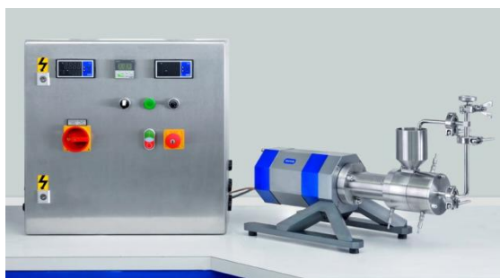
Figure 1: DYNO ® -MILL Model RESEARCH LAB
