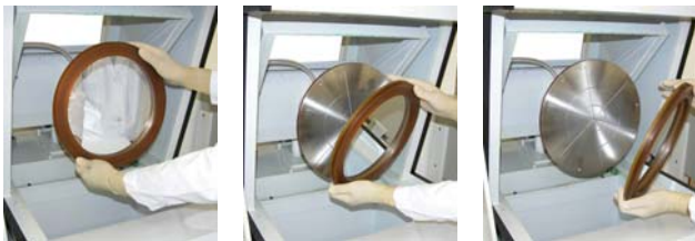
(Illustration 6) 300 mm vacuum rotating cathode backplate
