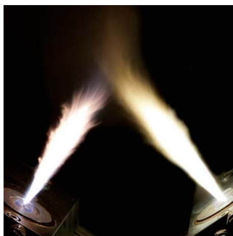
Figure 1: Photograph of the two-nozzle FSP setup as used for preparation of Pt/Ba/Al 2 O 3 catalysts. The Al and Ba particle streams are mixed after formation of individual Al 2 O 3 and BaCO 3 nanoparticles.
