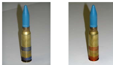
Figure 6. 50 Cal. Round After Exposure Over 157°F
