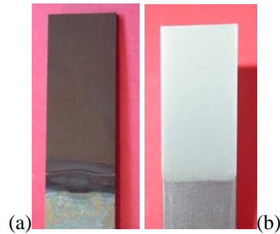
Figure 2 Micrographs of Ti alloy coated foils, (a) HAP-5wt%CNTs (b) HAP-0wt%CNTs
