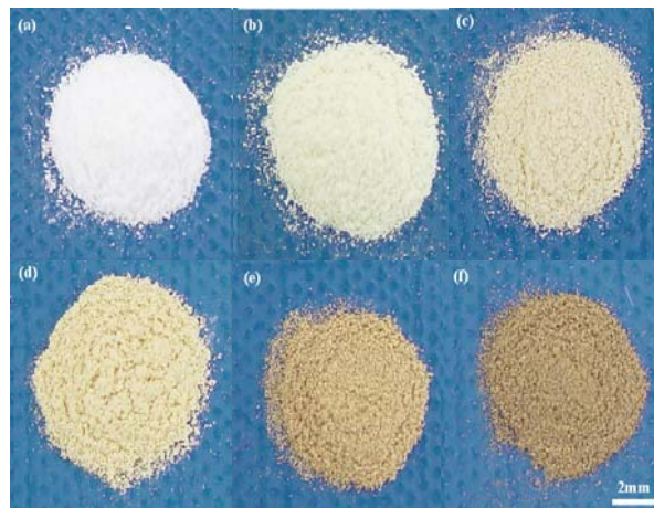
Figure 1: Optical images of pristine \text{Al}_2\text{O}_3 powder and Ag-deposited \text{Al}_2\text{O}_3 powders as a function of the deposition time; (a) pristine \text{Al}_2\text{O}_3 , (b) 150 min, (c) 390 min, (d) 550 min, (e) 770 min, and (f) 990 min.
