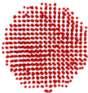
Figure 3: Arrangement of atoms in 3 nm Au particles. The particles appear with a moderately relaxed surface and a more densely packed interior/core divided into domains that are misoriented with respect to each other.
