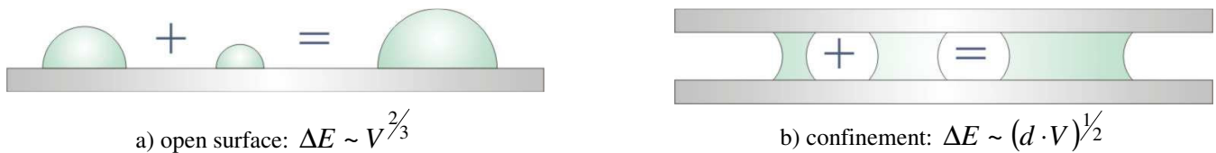
Figure 4: Reduction of the potential energy by the coalescence of two droplets.
