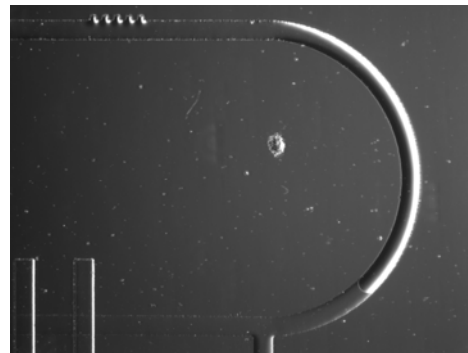
Fig. 3 A Micrograph of the PDMS channel with Gate-Controlled Valves
