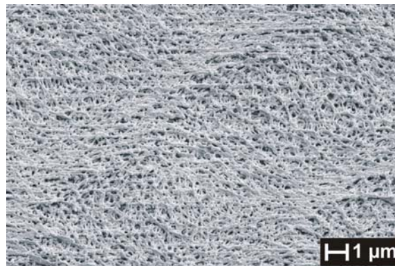
Figure 5: A nearly flat surface made by back-side exposure with nano pores below 500 nm.
