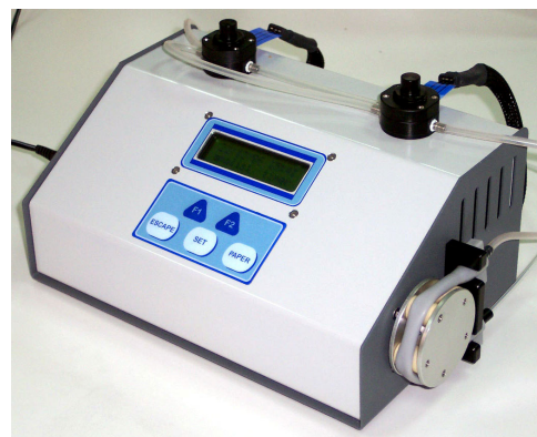
Figure 5: Photograph of the fabricated biosensor with two flow cells for biomediators in series.
