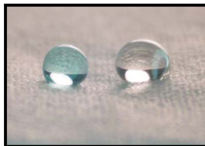
Figure 2: Water and oil (respectively shown) on a treated piece of fabric composed of cotton fibers.
