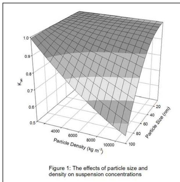
Figure 1: The effects of particle size and density on suspension concentrations
