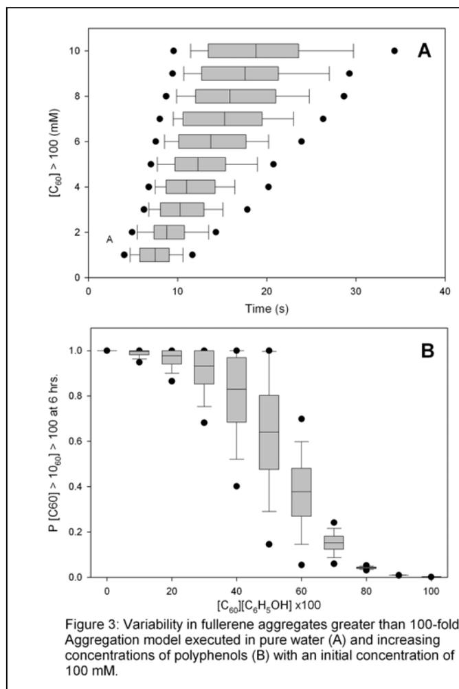
Figure 3: Variability in fullerene aggregates greater than 100-fold. Aggregation model executed in pure water (A) and increasing concentrations of polyphenols (B) with an initial concentration of 100 mM.
