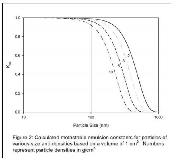
Figure 2: Calculated metastable emulsion constants for particles of various size and densities based on a volume of  $1 \text{ cm}^3$ . Numbers represent particle densities in  $\text{g/cm}^3$
