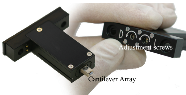
Figure 2: Cantilever array holder used with the Cantisens Research instrument. The holder allows fast sensor handling and adjustment towards the optical read-out.
