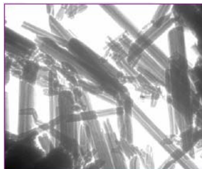
Figure 1. Halloysite clay nanotubes (200nm diameter)
