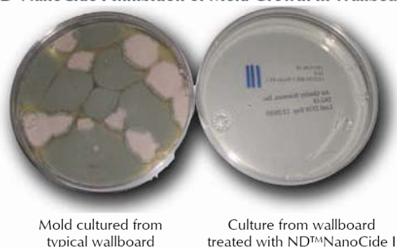
Figure 2. Inhibition of mold by wallboard paper treated with controlled release mold inhibitor.
