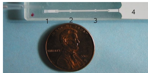
Figure 1: A prototype micro-lateral flow strip. 1 \mu l sample droplet shown applied to application pad (1), via pipette. Flow proceeds through detection pad (2) and control pad (3) to absorber pad (4).
