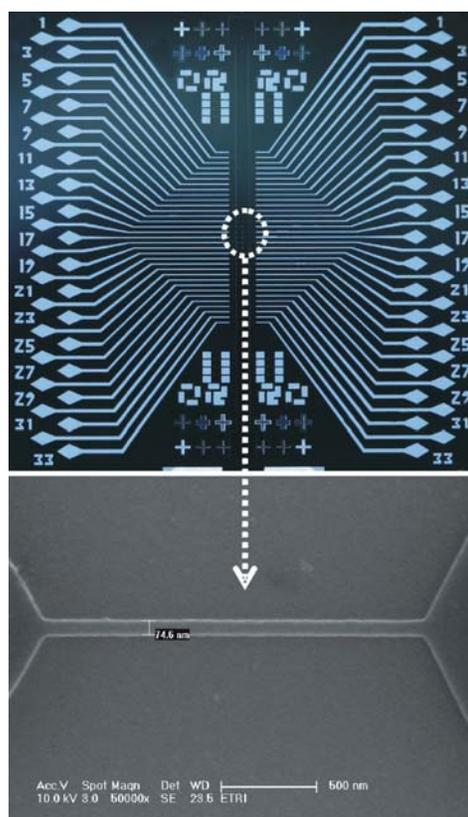
**Figure 1:** Structure of a Si FET nanosensor (2 cm  $\times$  2 cm). Right panel shows a SEM image of one out of 33 individual nanochannels, height: 40 nm, width: 75 nm.
