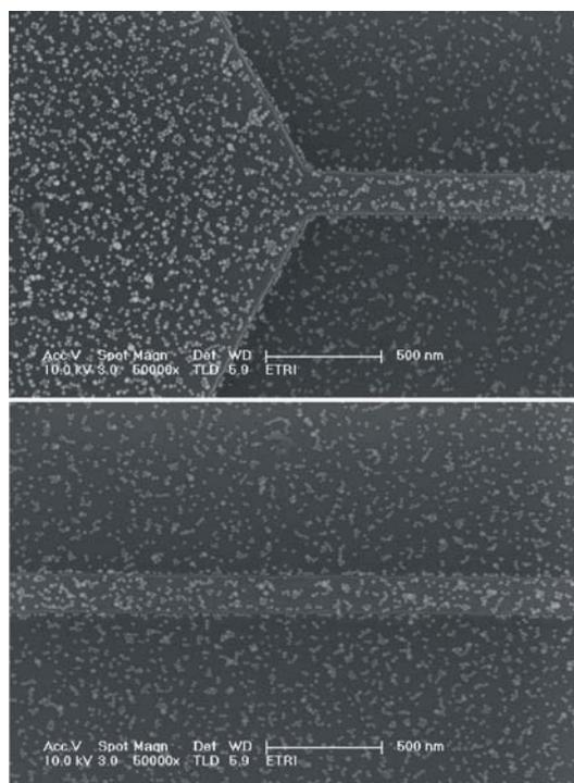
**Figure 2:** SEM images of nanochannels labeled by DNA derivatized-13 nm Au NPs. Particle density of nanochannels is about 1100/μm<sup>2</sup>.
