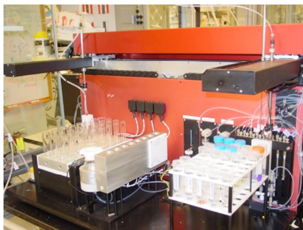
Figure 5. Custom robotic combinatorial peptoid synthesizer capable of fully automated mix & split library synthesis.
