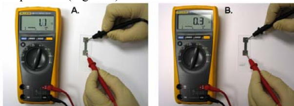
Figure 5. Resistance measurements of two silver fluids
