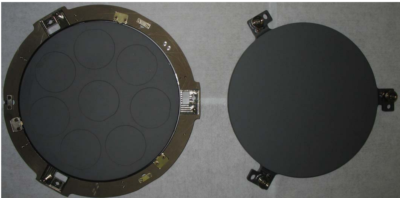
Figure 2: Left – Fixture base plate with outlines for 8 two-inch wafer pairs. Right – Fixture top plate
