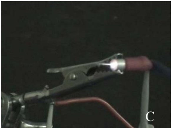
Figure 1. Representative firing pulses of 0.125-inch diameter solid-state gas generator using ECESP: A) Low power operation, B) high power operation, and C) Minimum power operation, capable of hundreds of discrete, reproducible combustion pulses using digital electric control.
