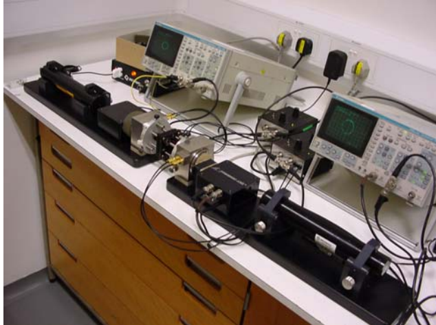
Figure 1: The two interferometer arms set up at NPL for a differential measurement.
