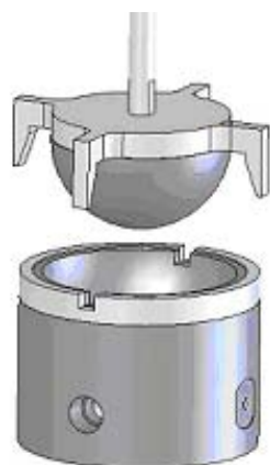
Fig. 2. Electrode (lower part) and cup implant holder fixture (upper part) for the porous hip substrate.
