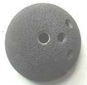
Fig. 4 Sintered HA/glass coated cup implant
