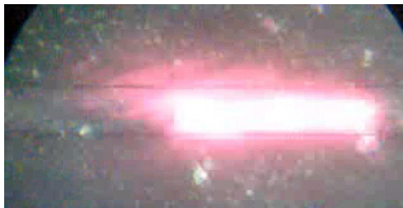
Figure 8. Laser-beam/driving bubble reaching centre of frame
