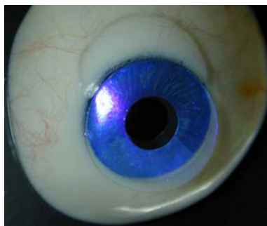
Figure 4. Photograph of the blue cosmetic lens prototype made of PCCA with the central transparent part. The prototype is placed on the artificial eye ball.
