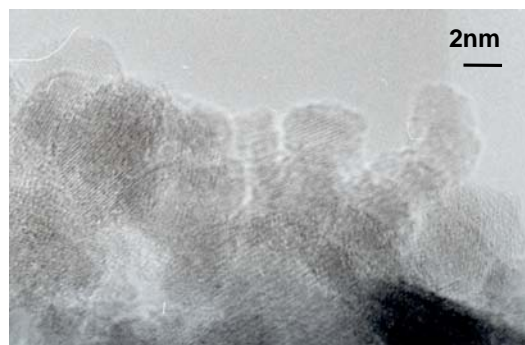
Figure 2: HRTEM image of the highly crystalline structure magnetite/ maghemite in silica.
