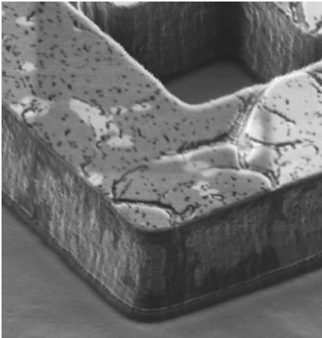
Figure 7: An SE image from the prototype helium ion microscope. The horizontal FOV is 5 \mu\text{m} . Note the fine topographic features which are evident.
