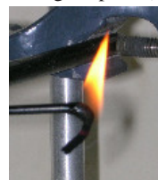
Figure 7 : Flame test on a HDPE/N9000 composites
